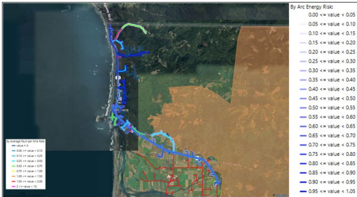
Figure 4.5-17: SR370 with zonal Faults per Mile Rate overlaid with zonal Arc Energy score
