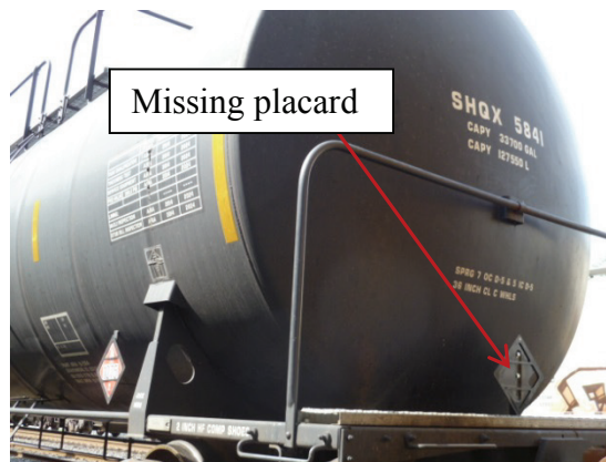
Tank Car (above) missing a hazardous material placard. Placards are required on all four sides of tank cars.
