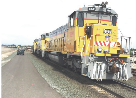
Photo at the west end of the UPRR Inbound JR Davis Yard in Roseville. There were no hand brakes applied on any of the three remote-control locomotives.
