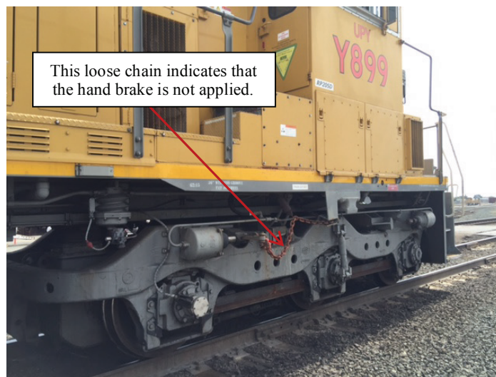
This lead locomotive, in addition to two coupled locomotives in the three-locomotive consist, was left unattended and unsecured with hand brakes.
