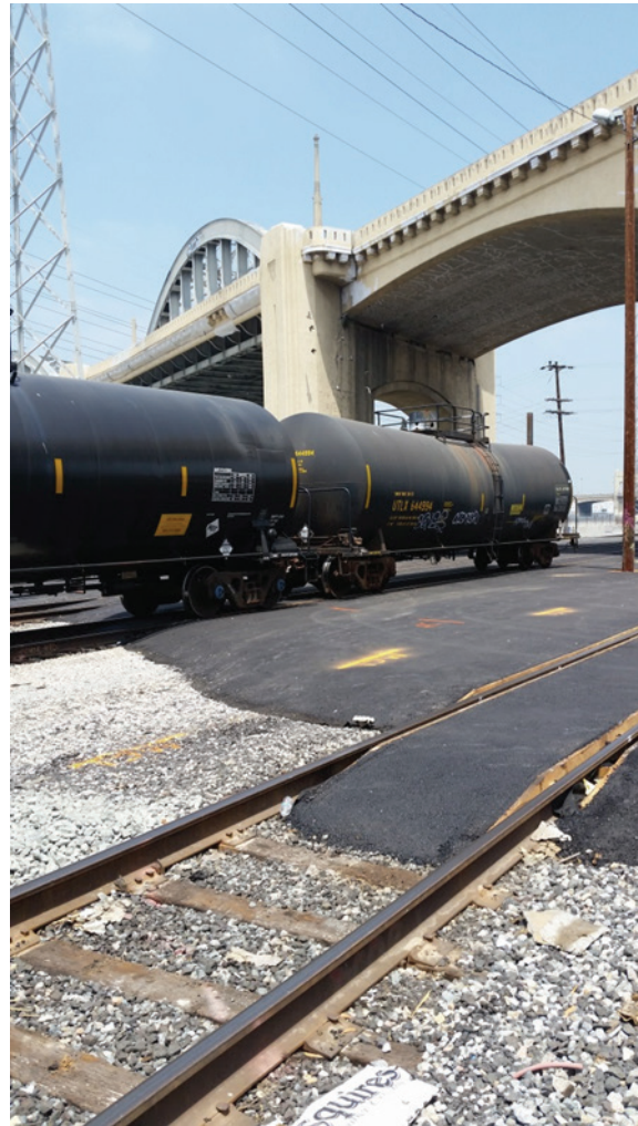
The UPRR 4 th Street Yard and 4 th Street Bridge; hazardous materials tank cars where the pavement was improperly applied.
