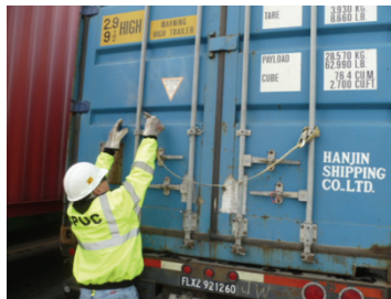
CPUC railroad safety inspector properly placing a "safety" strap to guard against a shifted load which could force the doors to open uncontrollably.
