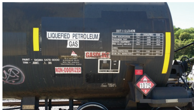
Example of improper commodity markings on a tank rail car. The placard number references gasoline (1075); however, the label states “Liquefied Petroleum Gas.” Both gasoline and Liquefied Petroleum Gas would not be shipped the same tank car. Firefighters would not know how to deal with the materials in the case of a derailment because both materials react differently when released.
