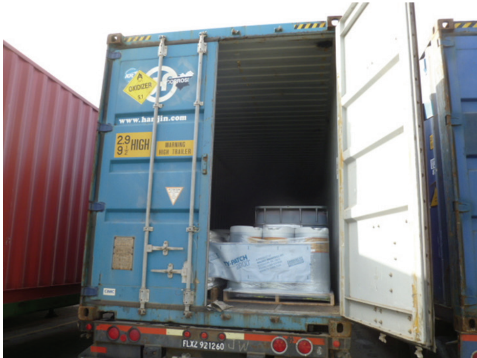
Observing an opened UP freight container. No defects were noted, as the materials were adequately blocked and braced according to regulations.
