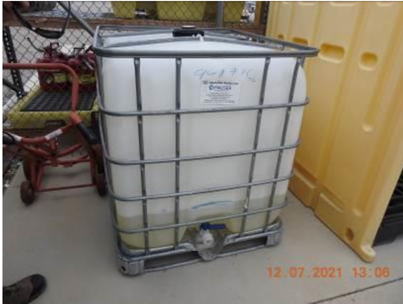
A container of liquid in the hazardous waste area without secondary containment.
