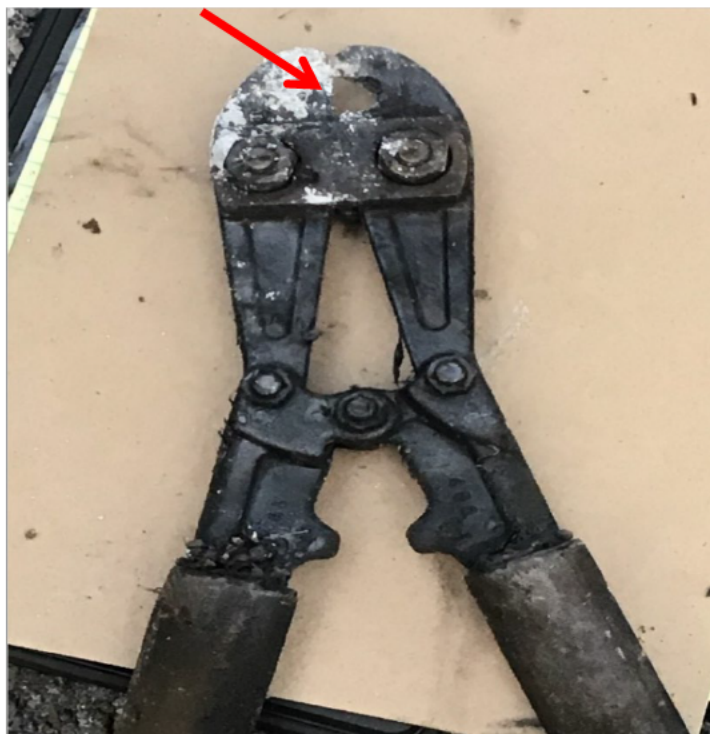
Figure 2: Bolt bite style cutters that made contact. The hole in the cutters (red arrow) was damaged when the cutter electrically connected the energized conductor and neutral.
