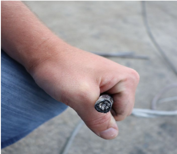
Figure 7: Disfigured conductor (supply side)
