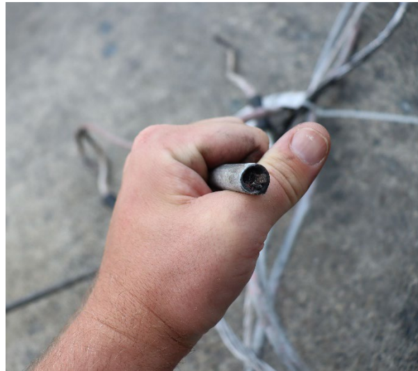
Figure 8: Disfigured conductor (load side)
