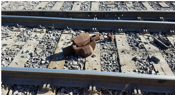
The broken coupler "knuckle" that failed between rail cars 32 and 33
