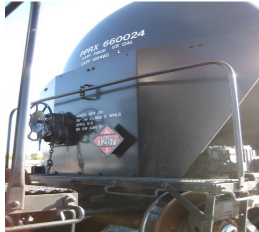
Crude oil tank car with enhanced or retrofitted material applied to the bulk head (end of car)
