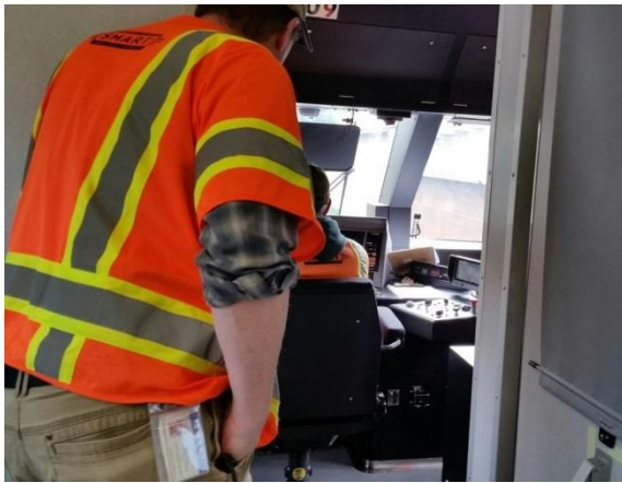
View of operator's cab of SMART PTC test train. The PTC console is a small, slim unit seen to the right of the operator.
