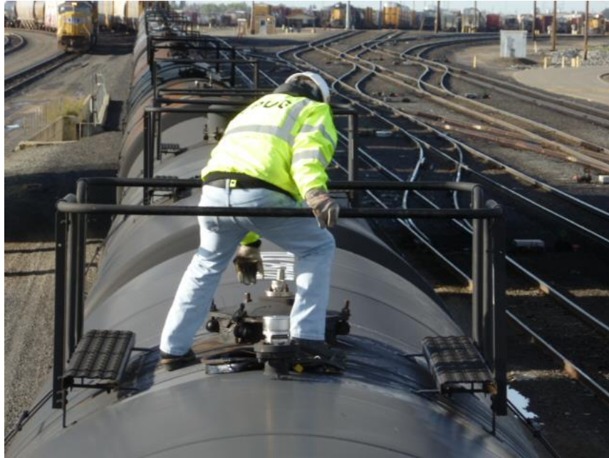
A CPUC inspector inspecting tank cars that carry hazardous materials for secure closures
