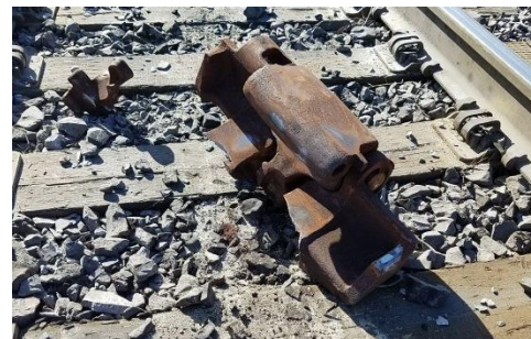
The broken coupler "knuckle" that failed between rail cars 32 and 33
