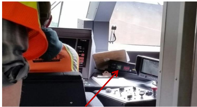
View of operator's cab of SMART PTC test train. The PTC console is a small, slim unit seen to the right of the operator.
