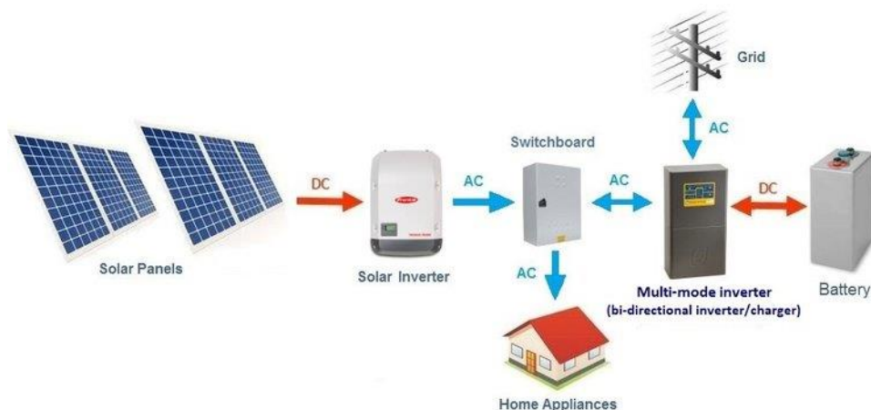
Figure 4 Example of AC-coupled DER System
